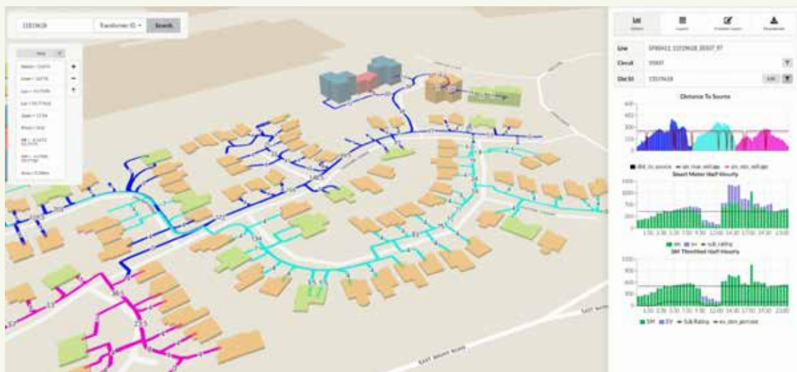
NAVI platform visualisation showing circuit connectivity, ADMD estimation and building understanding
