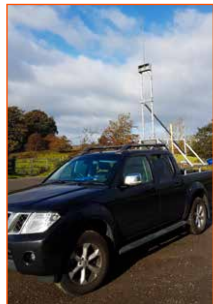
Figure 9 Mobile radio frequency receiving equipment used to detect arc-induced radio frequency signals
