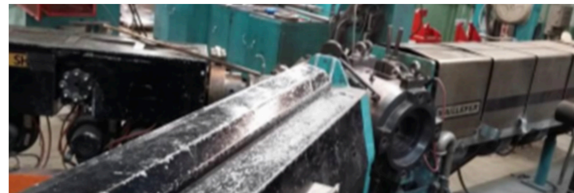
Figure 4 Picture showing the triple head extruder used in General Cable Silec's cable manufacturing of the MV Suscable core. The cable core then passes through a water bath cooling zone 80m in length with no crosslinking stage.
