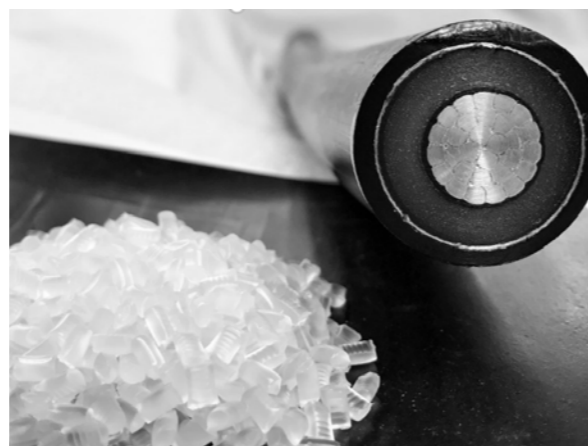
Figure 3 Picture showing the pelletised blend granules which are translucent with the corresponding extruded MV cable. The aluminium conductor has an adjacent black inner semiconducting screen and there is an outer screen bounding the insulation layer – this layer appears dark grey because the cross section acts as a black reflector.
