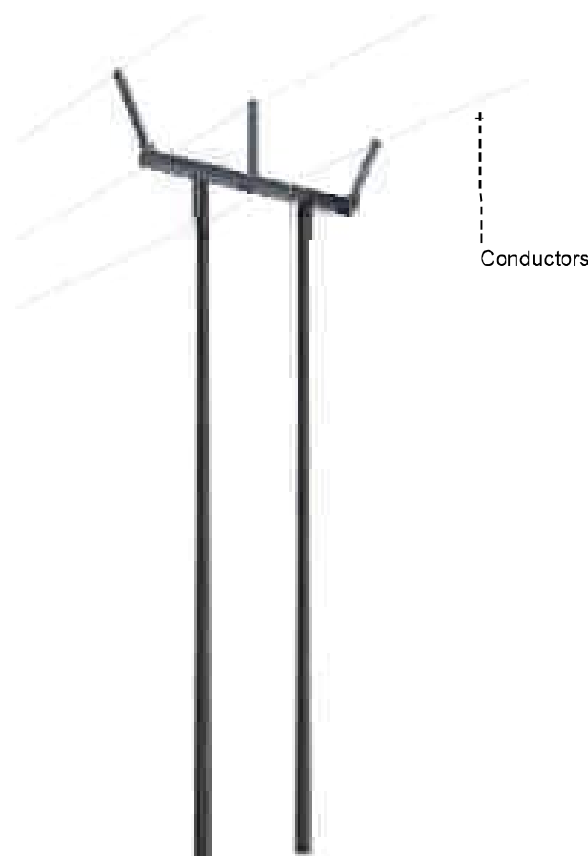
Component parts of 132kV 'Trident' design wood pole: Intermediate (H pole)
