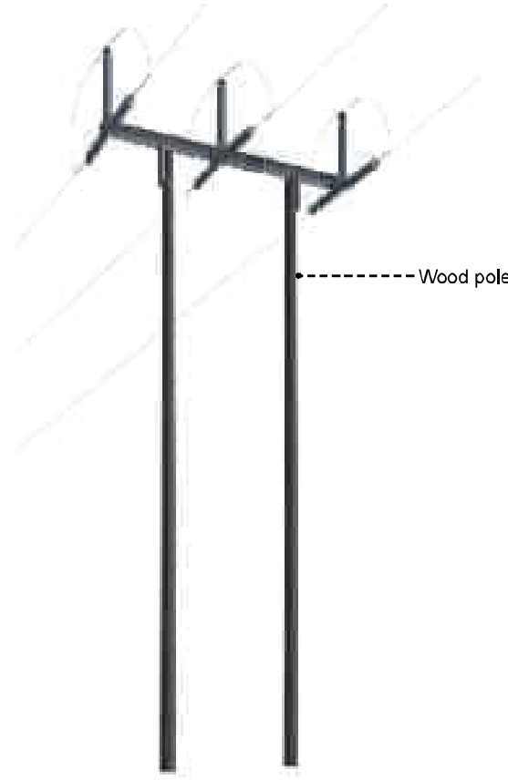
Component parts of 132kV 'Trident' design wood pole: Angle (H pole)
