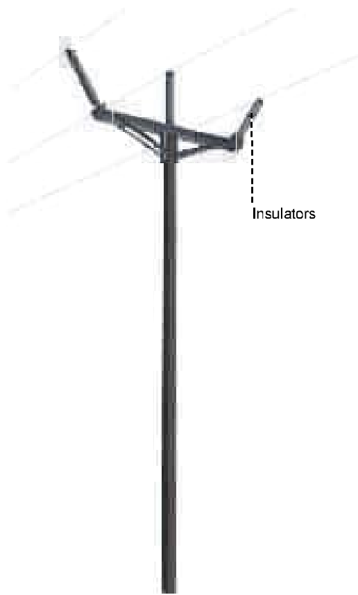
Component parts of 132kV 'Trident' design wood pole: Intermediate
