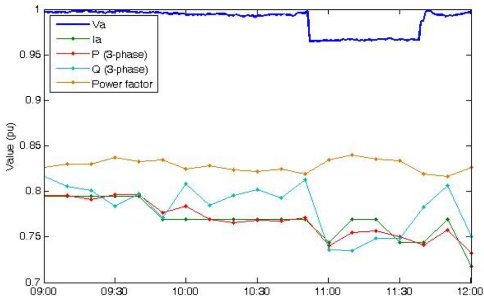
**Figure 4: Load at Cupar during Juniper voltage reduction**
