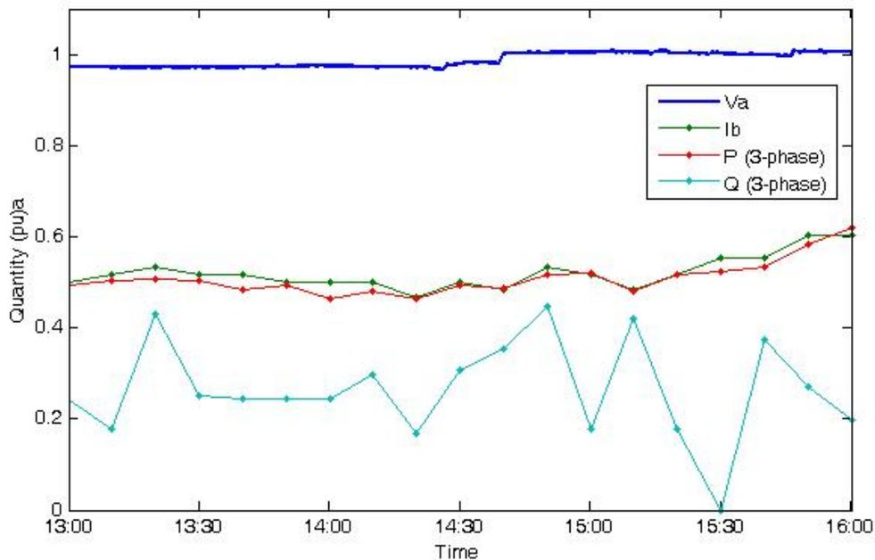
**Figure 8: Ruabon load at removal of voltage reduction**
