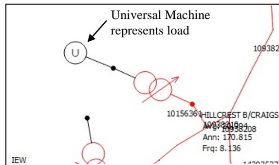
**Figure 9: Universal machine added to IPSA network model**
