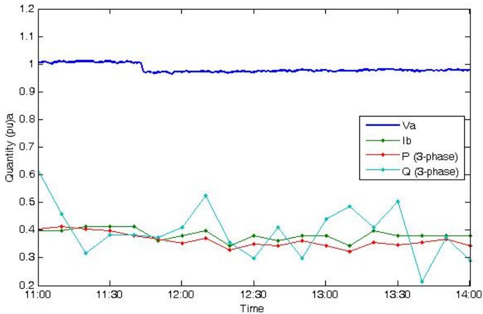
**Figure 7: Ruabon load at application of voltage reduction**
