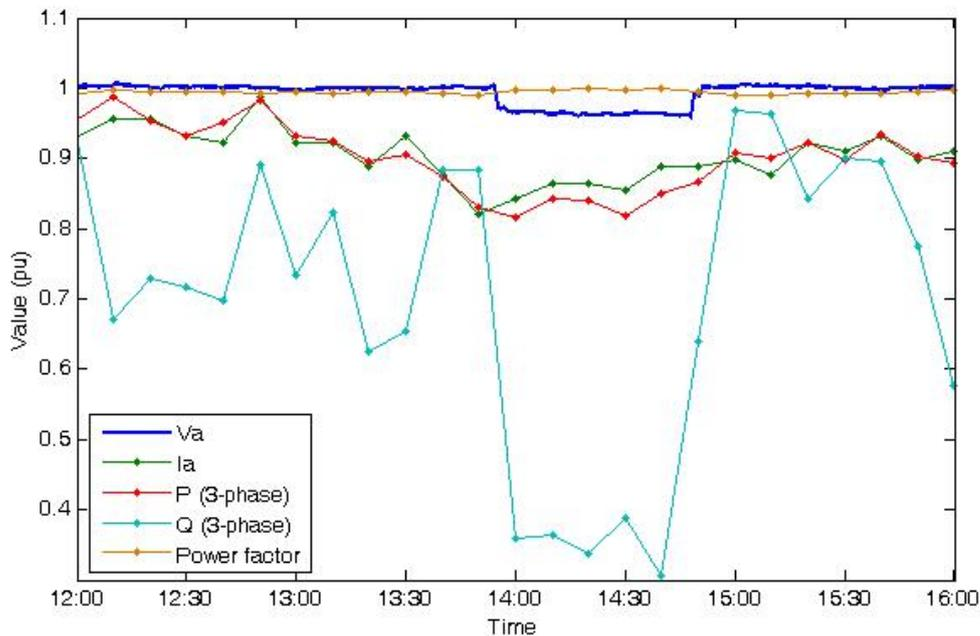
**Figure 5: Load at Liverpool Road during Juniper voltage reduction**
