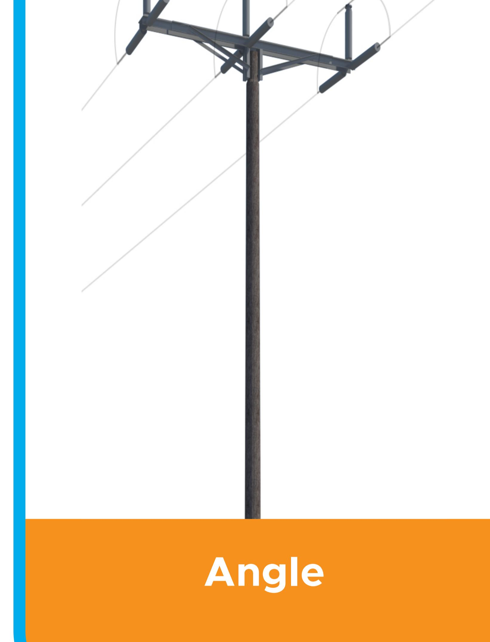
Wood poles have an average height of 14 metres, however this can be increased or reduced depending on the structure or features of the land.
