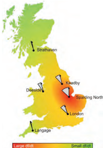
Figure 7 Regional RoCoF and angle deviation in response to a disturbance
