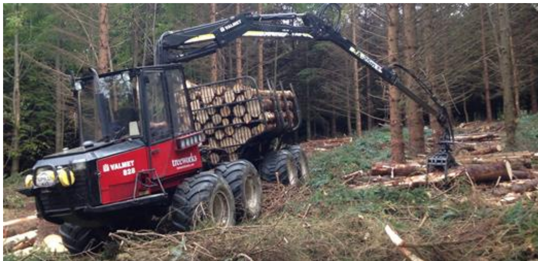
Photo 4.3: Timber Forwarding Vehicle
