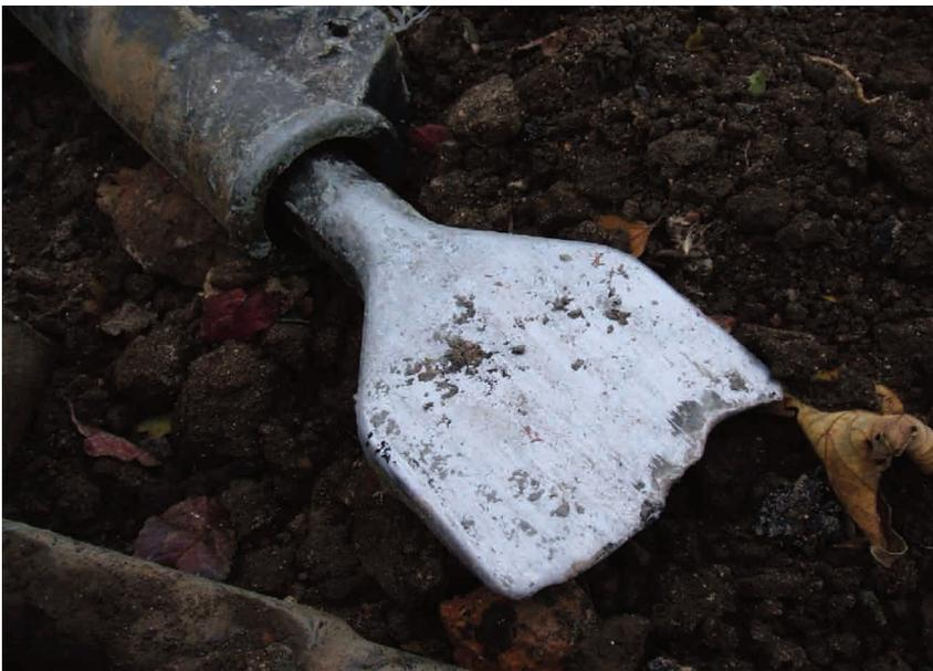
The above image highlights a damaged spade tool on a pneumatic gun which has come into contact with a low voltage cable.
