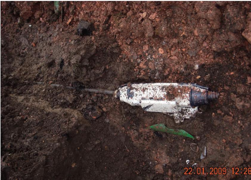
The above image highlights a low voltage cable with a straight joint attached. An operative took a hacksaw and severed the cable which was attached to the ScottishPower network.
