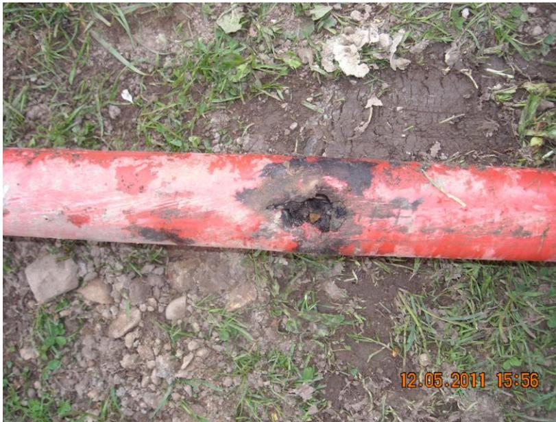
The above image demonstrates the impact on an HV cable when a 910mm long steel pin was driven into the ground.
