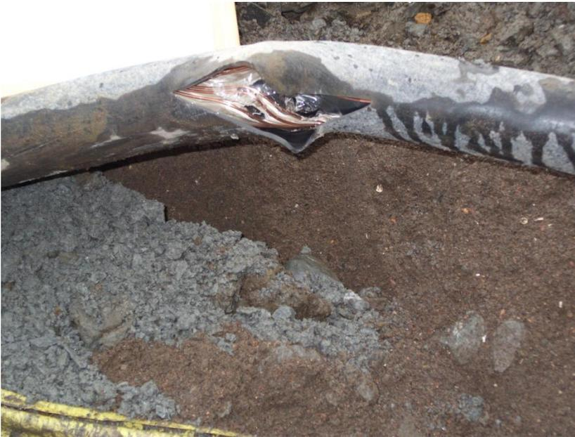
The above image clearly demonstrates the impact on the underground ScottishPower network, when an excavator came into contact with a low voltage cable (240 (4) Waveform)
